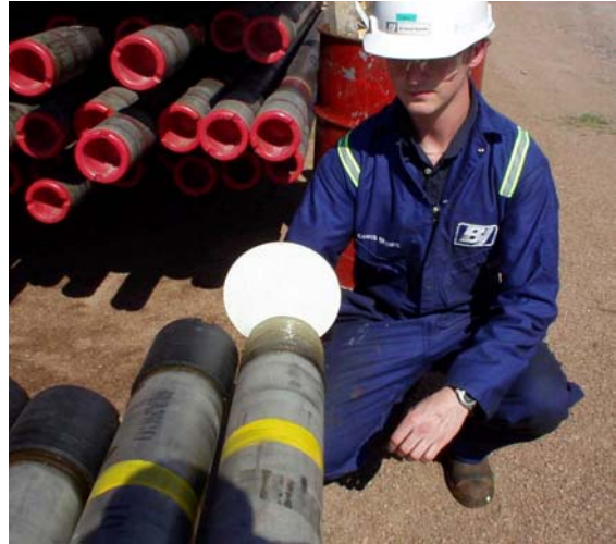
Stainless steel sleeves and stainless steel target plates are equipment available with the SpeedTally laser tally system.
